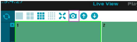
After the screenshot, the image will be opened using the Windows photo viewer and the saved path of the image will be displayed. The screenshot save path can be viewed or modified by setting SnapPic entries locally.
