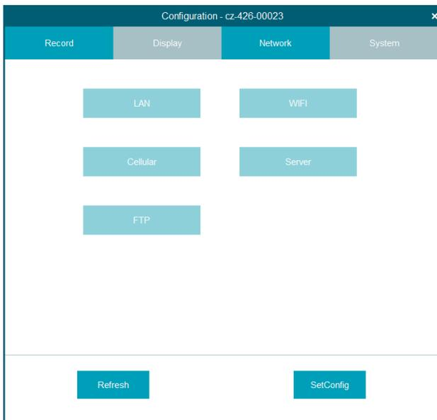
Through the network, you can check the LAN / WiFi / cellular / server / ftp status of DVR and modify the configuration of server / FTP.
